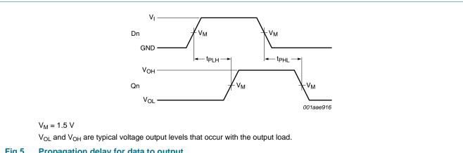
Propagation delay for data to output Fig 5.
